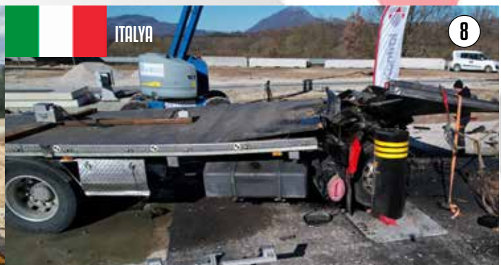
COUNTER TERROR FIXED BOLLARD 7500 KG / 80 KM
