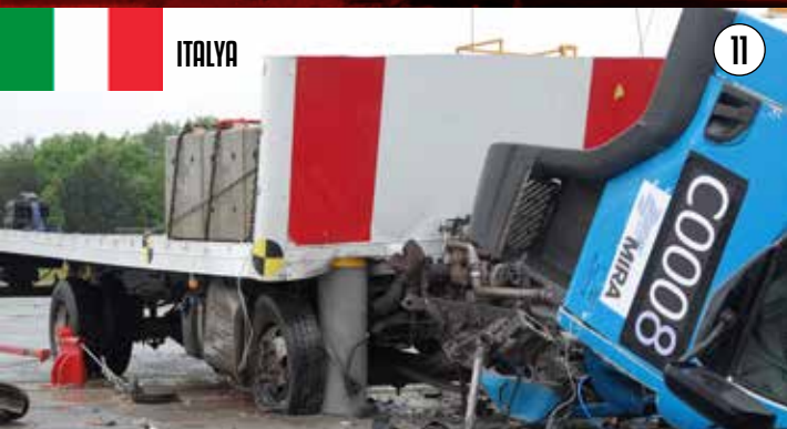
COUNTER TERROR FIXED BOLLARD 7200 KG / 48 KM
