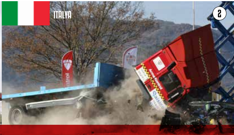
COUNTER TERROR RISING BOLLARD 7500 KG / 80 KM
