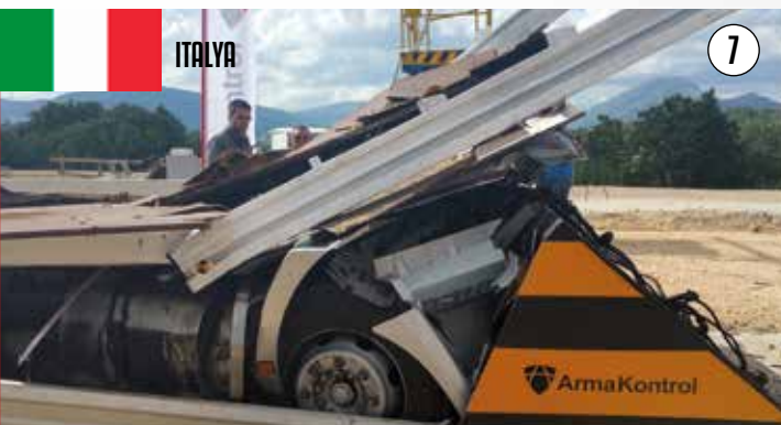
COUNTER TERROR ROAD BLOCKER 12000 KG / 80 KM
