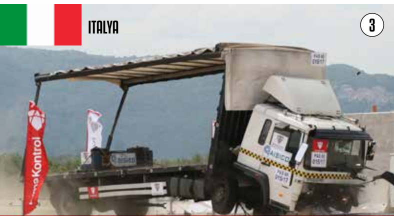
COUNTER TERROR RISING BOLLARD 7500 KG / 65 KM
