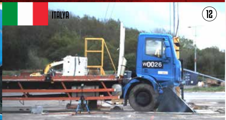
STANDARD ROAD BLOKER 7500 KG / 80 KM
