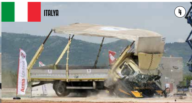
COUNTER TERROR TELESCOPIC ROAD BLOKER 7500 KG / 80 KM
